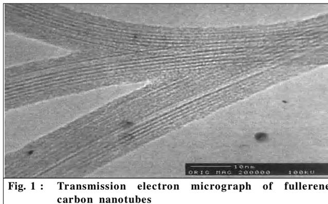
**Fig. 1 :** Transmission electron micrograph of fullerene carbon nanotubes
